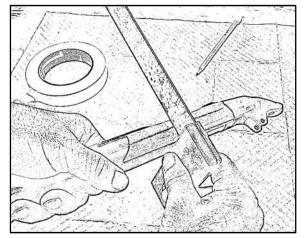
one limb of the square. It may help to roughen the edge of the square with sandpaper to hold the graphite. Place the square against the left side of the receiver with the graphite edge against the masking tape and the other edge flush with the flat bottom of the receiver. Rub the square back and forth on the masking tape to mark the center line of the side of the receiver.
